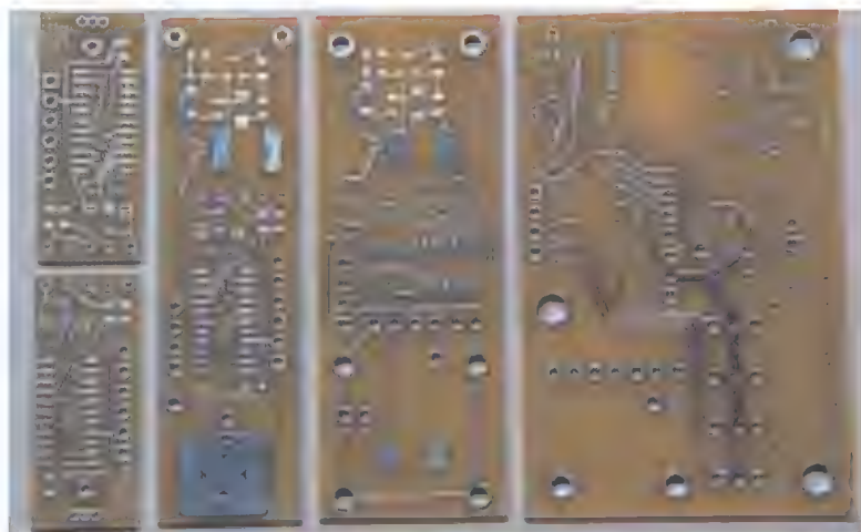
■ FIGURE 2. MiniBoard cut apart into individual flight computer boards.
